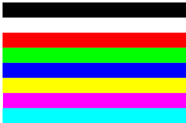
Figure 12-20 Horizontal Color Bar Test Pattern
